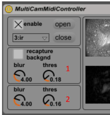
Figure 5. Pre-processing (1) and post-processing (2) blurring and thresholding parameters
